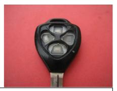
Using flat screwdriver gently lift up and shave off worn rubber layer consisting of key buttons. You can use Stanley knife to cut it smooth around the edges. Be careful not to cut too deep to avoid damaging plastic shell. You should end up with remote looking like the one on the right hand side ready for inserting new buttons in.
