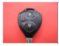
The most common fault of Toyota remote that suit: Hilux, Rav4, Yaris and many other models is deteriorating rubber key pad. This rubber pad is an overmolded part of the plastic shell and over period of time it becomes brittle and cracks.
